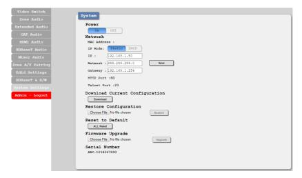
■ **Power:** Press this switch to toggle the unit's power between ON and OFF (standby mode).
