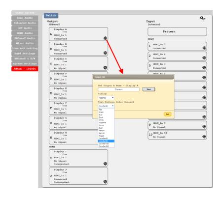
■ **Test Pattern Colour Control:** The test pattern type can be changed to any one of sixteen different options. The patterns include full screen colours as well as a selection of other basic patterns.
