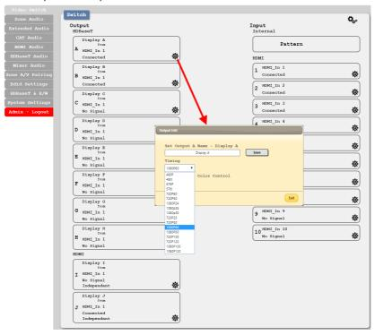
■ **Timing:** Test patterns can be generated on either the HDMI or HDBaseT outputs at the following standard resolutions with a variety of refresh rates: 480i/p, 576i/p, 720p, 1080p, 4K. Test pattern output does not enable HDCP.
