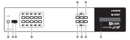
1 POWER BUTTON: Press this button to power the unit on or place it into stand-by mode.
