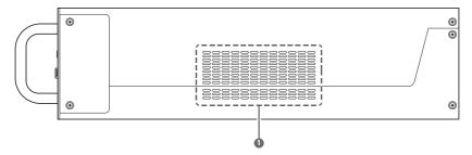
**1 VENT FAN:** These vents are for are for air ventilation. Please allow adequate space around the unit for air circulation.
